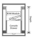
The KVM Module can be connected to a console, or be used as a stand-alone KVM Switch. There are three major categories: PS/2, USB and Sun Interfaces.
